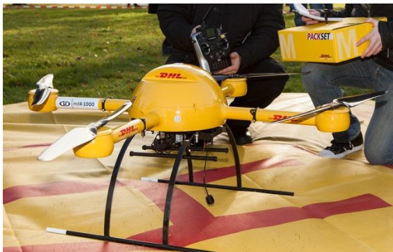
Figure 5 - md4-1000 drone testing for DHL package delivery Image courtesy of Author Frankhöfner and Wikipedia
