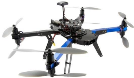
Figure 13 - Top of the X-8 showing motor booms and landing skids Image courtesy of 3DR
