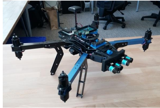
Figure 45 - The drone configured for the Arduino and Drone control testing phase, wiring not yet installed
