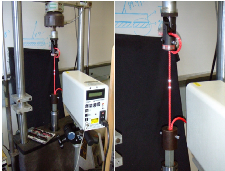
Figure A6.2.1- Rope Stretch Testing Apparatus
